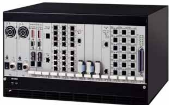
Figure 7. NEBS-Compliant Megaplex-2100 Chassis
